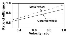
Fig. 1 Turbine efficiency of ceramic wheel and metal wheel
