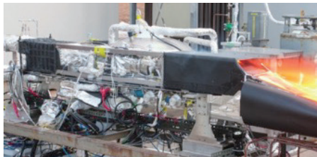
Precooled Turbojet Engine (Courtesy of JAXA)
