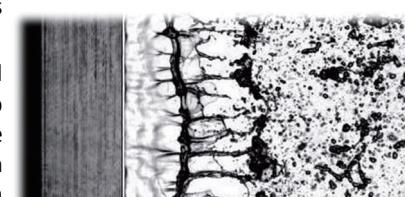
High-speed visualization of a planar liquid sheet fragmentation by high speed gas streams
