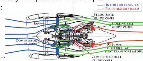
An intercooled and recuperated (ICR) turbofan using component heat exchangers and heat transport medium with the same weight of the baseline turbofan
