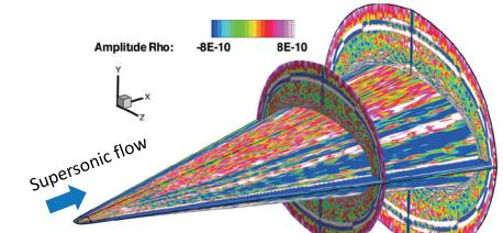
A computed result of eigen mode of density for the maximum eigenvalue around a sphere-cone flight model
