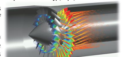
Total Pressure Distribution due to Rotor/Stator Interaction for Sound Pressure Evaluation using CFD
