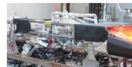
Precooled Turbojet Engine (Courtesy of JAXA)
