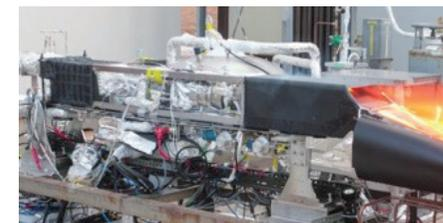
Precooled Turbojet Engine (Courtesy of JAXA)
