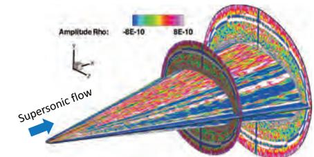
A computed result of eigen mode of density for the maximum eigenvalue around a sphere-cone flight model
