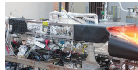
Precooled Turbojet Engine (Courtesy of JAXA)
