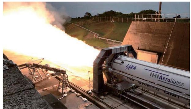
Fig. 5 SRB-3 firing Test
