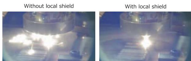
Fig. 5 Differences during Ti-6Al-4V printing with and without local shield
