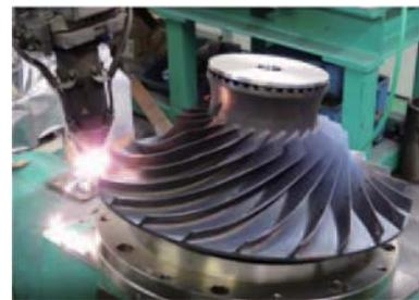
Fig. 11 Repairing of impeller by LMD
