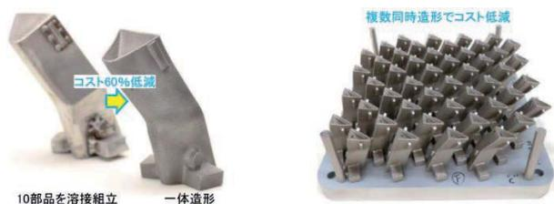
Fig. 14 Cost reduction by parts integration using AM
