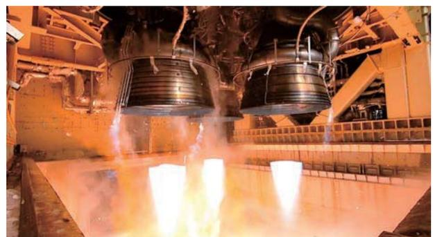
Fig. 8 First stage battleship firing test
