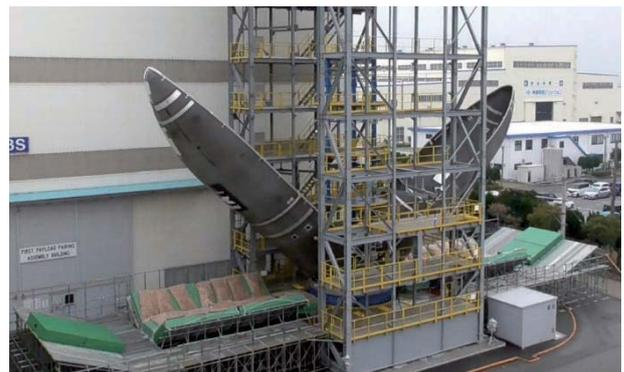
Fig. 6 Fairing separation test
