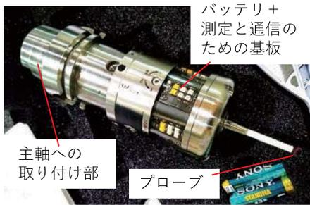
Fig. 6 Touch trigger probe
