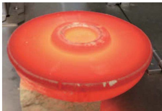
Fig. 7 Image of P/M disk forged with high-strain rate and intermediate temperature by NIMS 1500 ton forging
