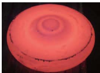
Fig. 10 Example of forged material(approx. \phi 550mm) with shape and size equivalent to actual disk material.
