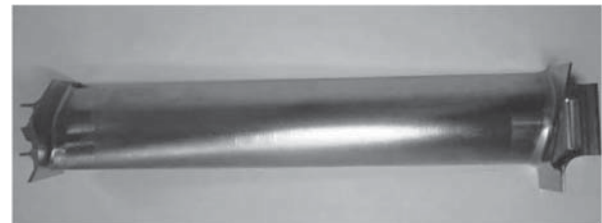
Fig. 7 Titanium aluminide low pressure turbine blade for GENx (3)
