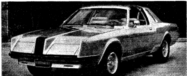
TURBINE CONCEPT car with a new dramatic aerodynamic design to go with the Upgraded Engine has been built for the U.S. Department of Energy by Chrysler Corp. The base car, a Chrysler LeBaron, was restyled as shown. Photo obtained by Bob Harmon at DOE Contractors meeting.
