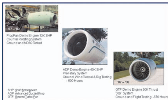
Illustration 7: Alternate Engine Arrangements Over Twenty Years of Technology and Cycle Development
