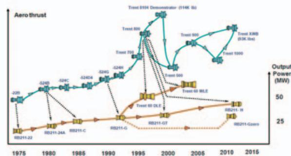
Figure 3 Aero engine origin of the Industrial RB211 and Trent
