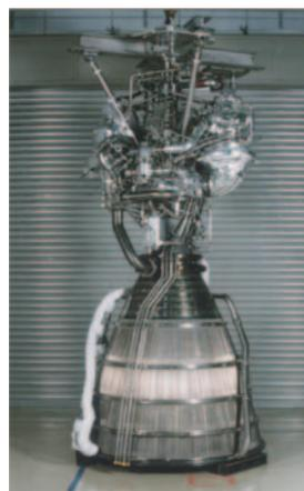
Fig. 1 LE-7A engine of H-IIA/ H-IIB launch vehicle
