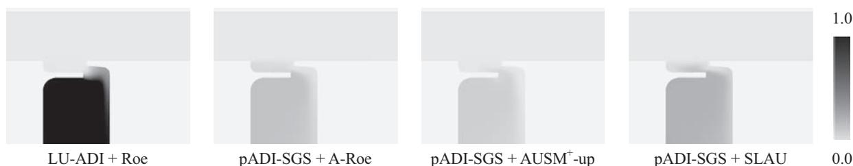
Fig. 3 Comparison of Seal Efficiency by Each Schemes
