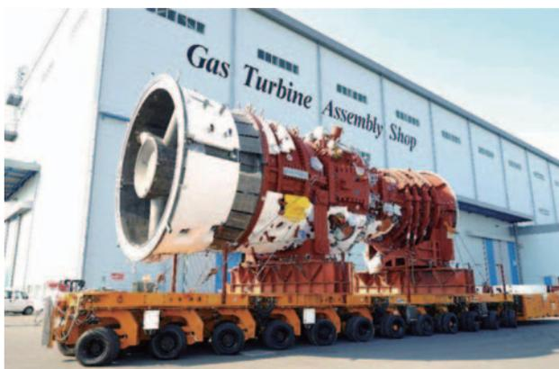
Fig. 2 1,600°C J-type gas turbine
