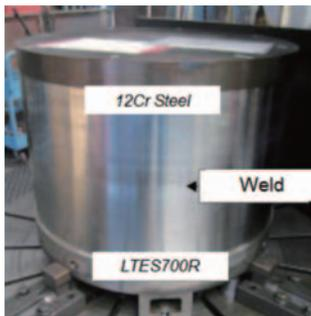
Fig.17 Rotor Dissimilar Welding<sup>(9),(10)</sup>
