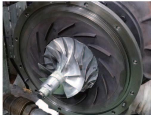
Fig. 2 Centrifugal compressor
