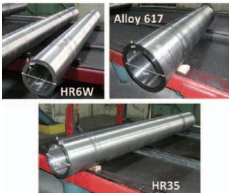
Fig.10 Boiler Pipes<sup>(2),(3)</sup>
