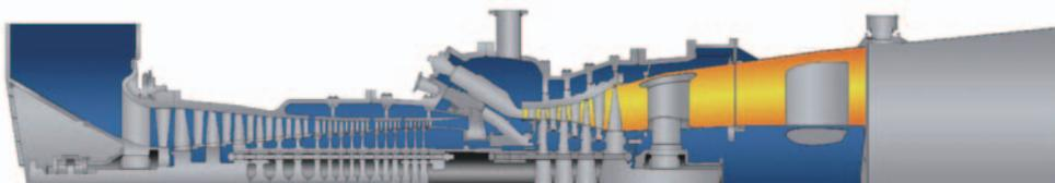
Fig. 7 Sectional view of M701F4 gas turbine
