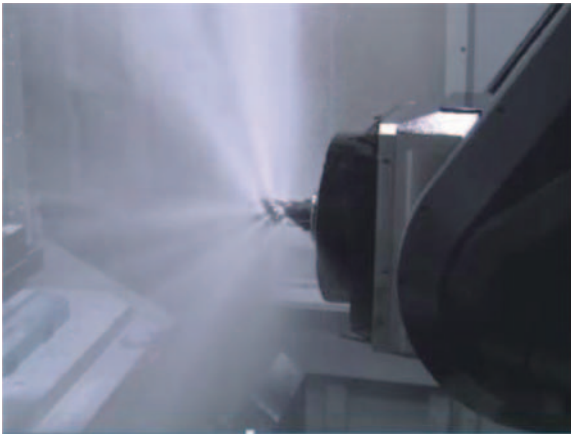
Fig. 7 High pressure and high flow through spindle coolant
