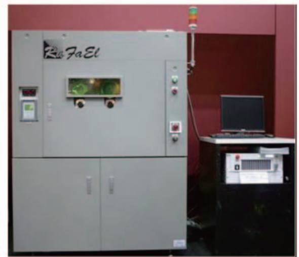
Fig. 2 Prototype system of selective laser melting system in vacuum condition. Developed by ALPROT, ASPECT and AIST (8)
