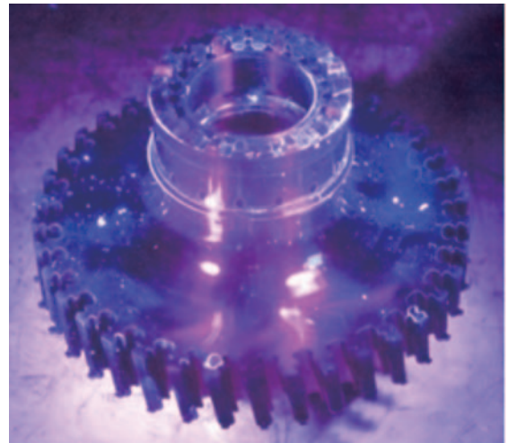
Fig. 9 Fluorescent penetration inspection of the gas generator turbine disk
