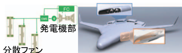
Fig. 4 Hybrid propulsion system and reference vehicle.
