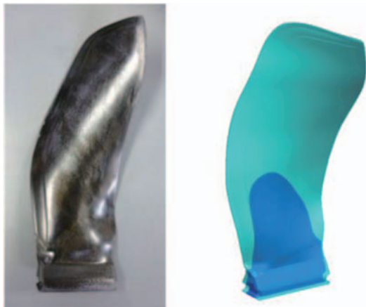
Fig. 3 Prototype of a hollow CFRP blade model and its CAD model.
