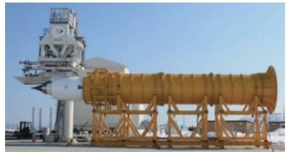
Fig. 7 Reverse endurance test (Outdoor test stand)
