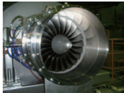
Fig. 5 Fan rig for aerodynamic performance test.
