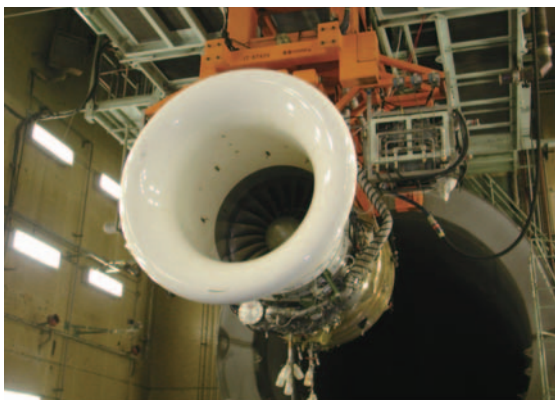
Fig. 6 Endurance test (Ground test cell)
