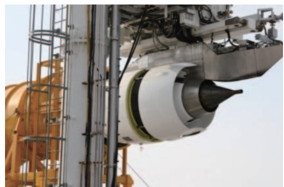
Fig. 8 Reverse endurance test (Max reverse)
