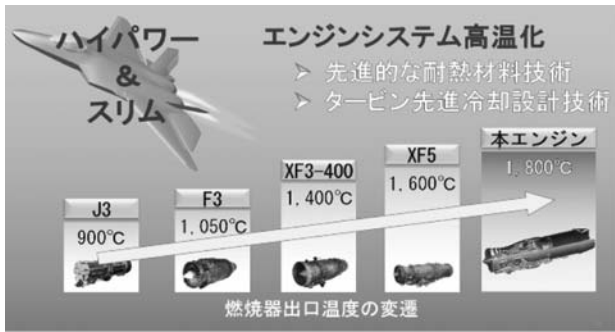
Fig.10 Step up of combustor exit temperature
