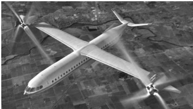
Fig. 7 Conceptual view of LCTR2 (the NASA Large Civil Tiltrotor) (14)
