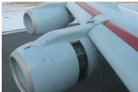
Fig.11 XP-1 full thrust reverse (Inside engine)
