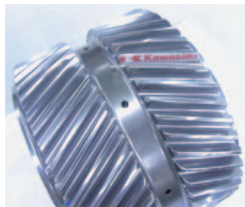
Fig.20 Gear Tooth Surface Super Finish
