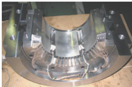
Fig. 2 Test tilting pad journal bearing
