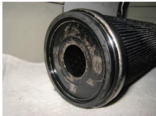
Fig. 6 Oil Filter used with blackened oil (Exxon Mobile MJ0254)
