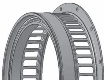
Fig. 9 Unitized model of a bearing
