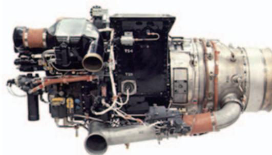
Fig. 10 Honeywell GTCP331-200 APU for Boeing 767
