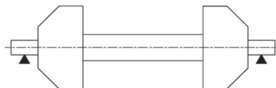
Fig.15 External bearing arrangement
