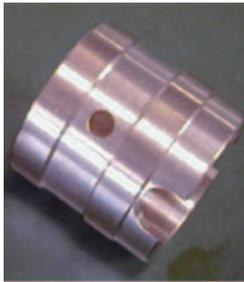
Fig. 7 Semi-floating bearing
