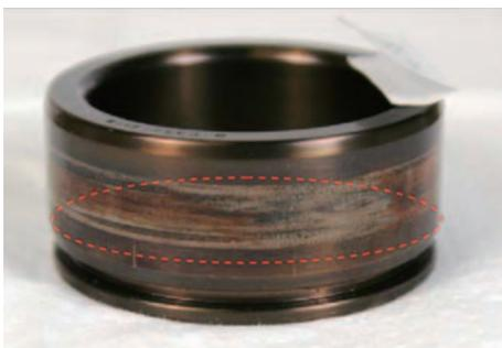
Fig. 7 Skidding damage
