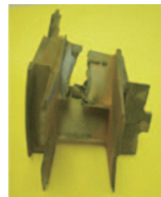
Fig. 6 Damage of high-temperature oxidation in vane
