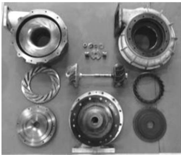
Fig.18 Parts of AT14 turbocharger
