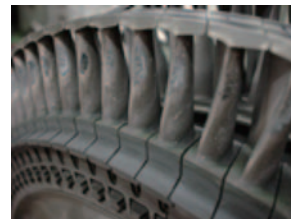
Fig. 5 Thinning of high-temperature oxidation in blade
