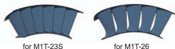
Fig. 7 Comparison of 4th turbine nozzle for preceding M1A-23S and for latest M1T-26
