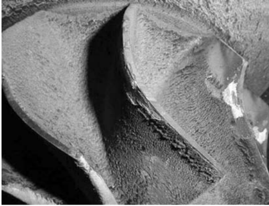
Fig.13 Deposit at turbine impeller
