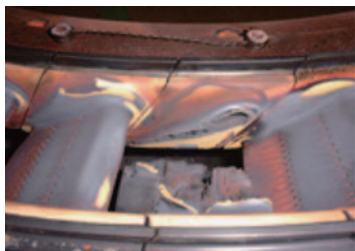
Fig. 7 Damage of high-temperature oxidation in vane
