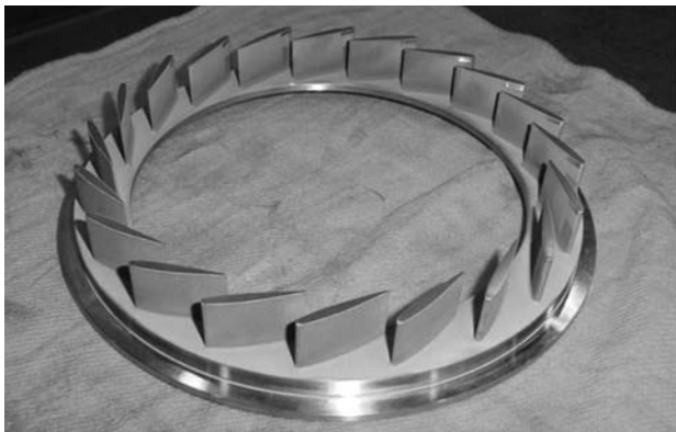
Fig.14 Nozzle ring with thermal spray coating
