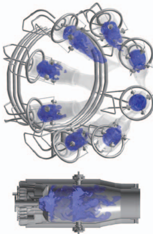
Fig. 1 Instantaneous iso-surface of gas temperature for whole (top) and one (bottom) combustor.
