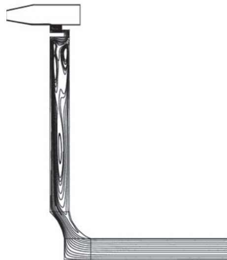
Fig. 12 Computed stream line pattern in the rotor-stator cavity
