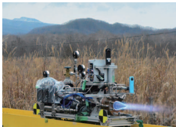
Fig. 10 Sled test of a rotating detonation engine (Kato et al. [12] ).
