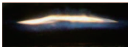
Fig. 13 Counterflow premixed n-decane-spray combustion ( \phi=0.85 , d_{32}=101\text{ }\mu\text{m} ) [6] . The premixed spray is supplied from the lower side and air is supplied from the upper side.
