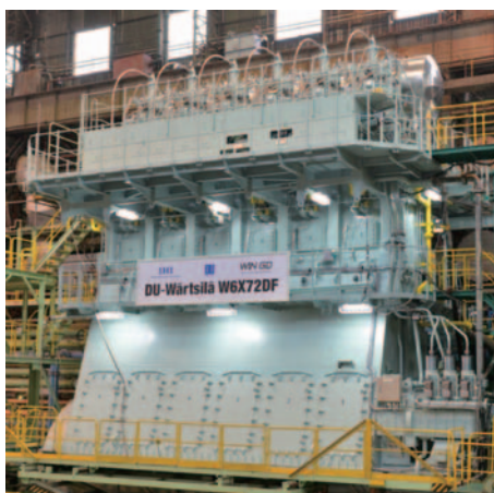
Fig. 6 Low-speed two-stroke lean-burn test engine (Bore: 720 mm · 19,000 kW · 89 rpm) (Diesel United, LTD. (1) )
