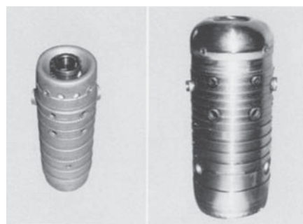
Fig. 4 Models of high-pressure combustor (left) and medium pressure reheat combustor tested in NAL (Not scale)
