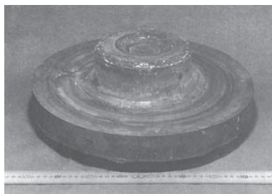
Fig. 3 Superalloy turbine disc as forged superplastically, using powdered alloy after HIPing (diameter : 340mm)
