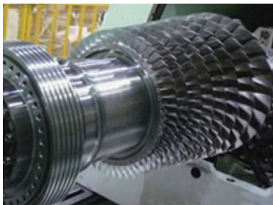
Fig.11 Schematic of the front 8 stages compressor test rig
