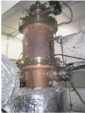
Fig. 15 Over view of the gas turbine combustor
