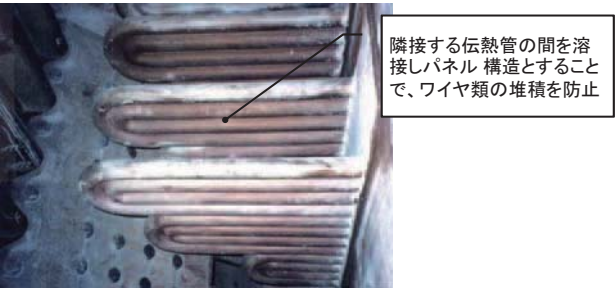
Fig. 4 Plate-shaped Heat Transfer Tube in Fluidized-bed
