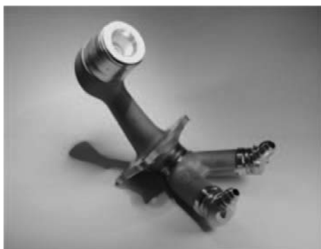
Fig. 15 A 3D-printed fuel nozzle for GE's LEAP 1-A engine 20)
