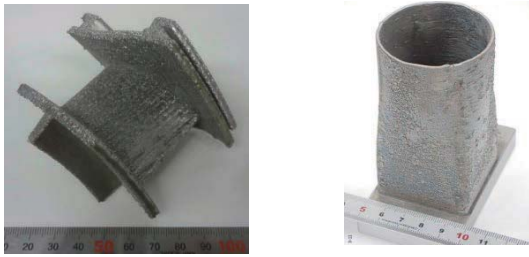
Fig. 13 Trial samples made by TRAFAM additive manufacturing machine (5), (6)
