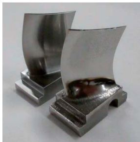
Fig. 5 Stators made by conventional manufacturing (back) and by additive manufacturing (front)
