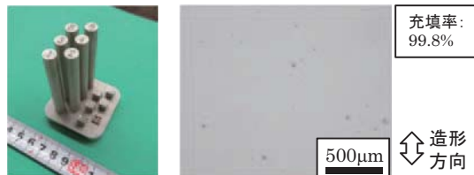
Fig. 6 Test pieces of alloy738LC and optical micrograph of test piece cross section
