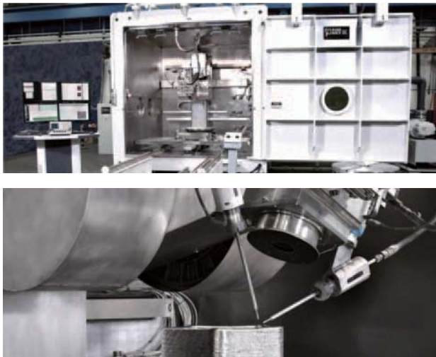
Fig. 13 Wire electron beam additive manufacturing system (4)
