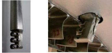
(b) Outlet total pressure and temperature probe for compressor
