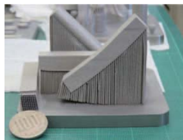
Fig. 1 Examples of fabrication failure of Ti-6Al-4V specimens by selective laser melting (SLM).
