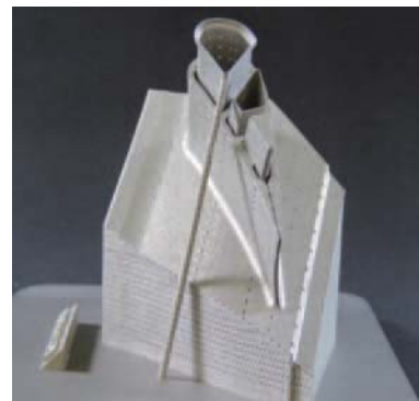
Fig. 5 MHA3300 Trial part (reduction model of gas turbine nozzle)
