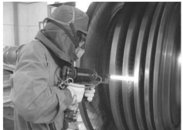
Fig. 11 HVOF coating on rotor surface
