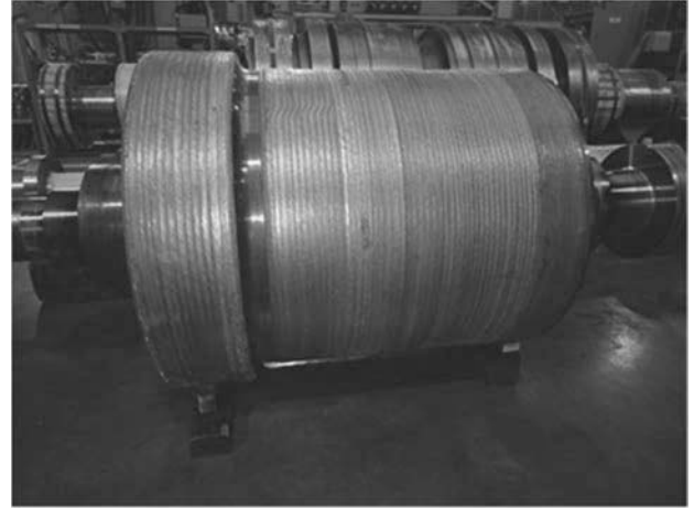
Fig. 10 Overlay welding on rotor surface
