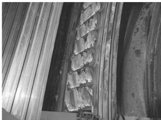
Fig. 13 Scale on stationary blade
