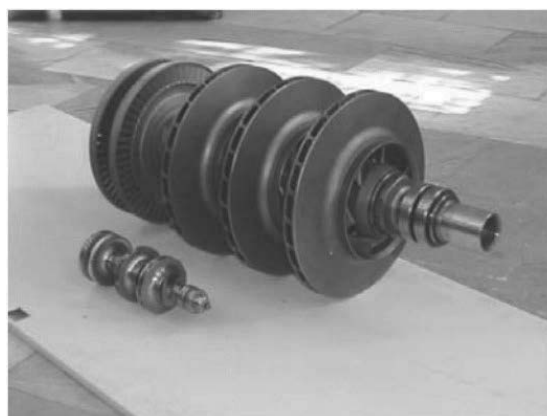
Fig. 8 RD-0120 and RD-0146 engine hydrogen pump rotors (14)
