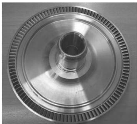
Fig. 7 Vulcain disk with integrated blades made by patented EDM method (12)
