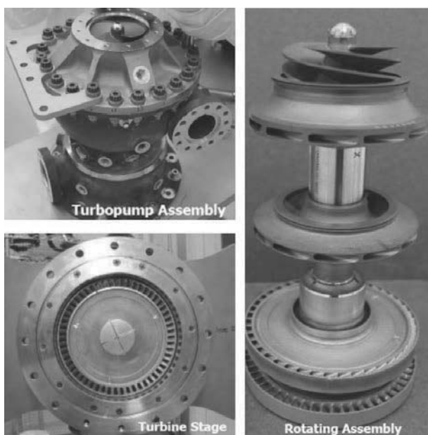
Fig. 9 Fuel turbopump of additive manufacturing demonstrator engine (16)
