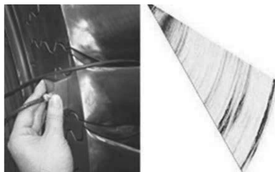
Fig. 14 Crack examination by phased-array ultrasonic testing method
