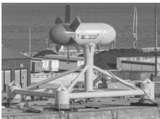
Fig. 12 The tidal power turbine of the Sabella. (14)
