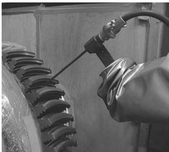
Fig. 12 Shot peening applied to blade grooves
