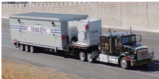
Fig. 16 30MW class mobile power FT8 Mobilepac
