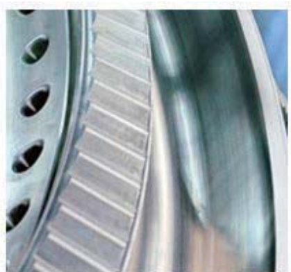
Fig. 6 Hirth Serration Design
