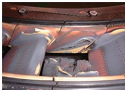
Fig. 4 Damage of high-temperature oxidation in vane
