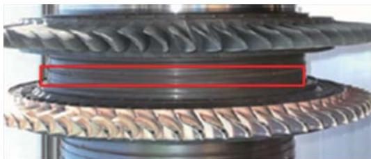
Fig.19 Incorporation state of air seal plate
