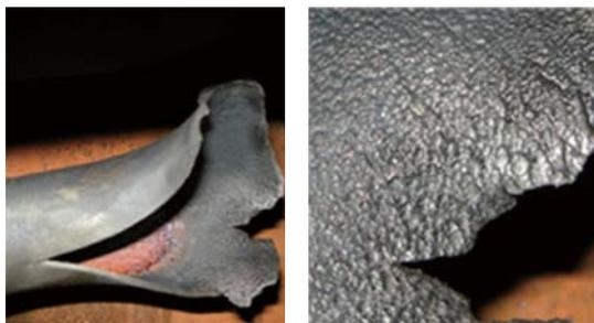
Fig. 22 Damaged tube and magnified photo of damaged area
