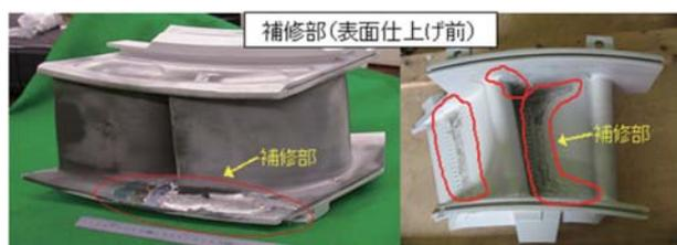
Fig. 10 Nozzle applied diffusion-braze repair<sup>(4)</sup>
