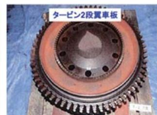
Fig. 17 Dirt inside the turbine disk
