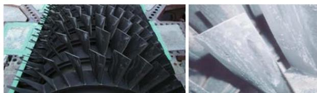
Fig. 7 Compressor appearance in inspection before the HEPA filter introduction
