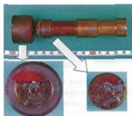
Fig. 16 Breakage of bolt
