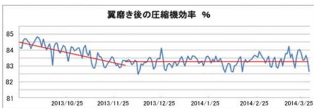
Fig. 12 Changes in compressor efficiency due to vane polishing
