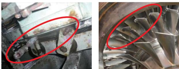
Fig. 11 Damage to the compressor due to disconnection of the linkage
