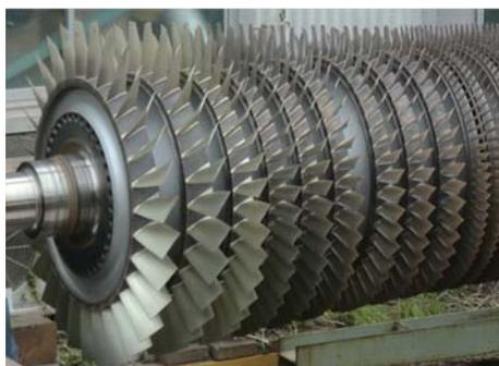
Fig. 8 Compressor appearance in inspection after the HEPA filter introduction
