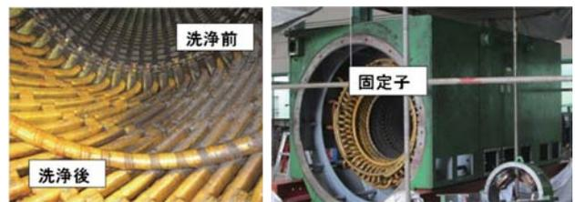
Fig. 21 Cleaning the generator stator
