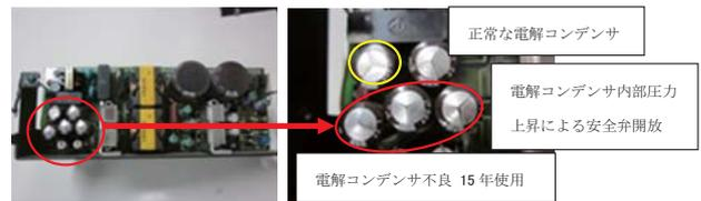
Fig. 25 Aged deterioration of condenser
