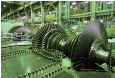
Fig. 15 Installation of new low-pressure rotor
