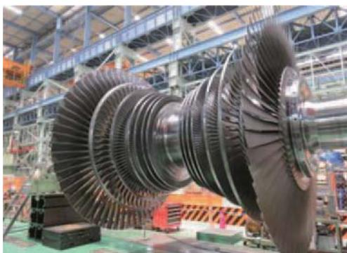
Fig. 11 New low-pressure rotor for Noshiro No. 1 unit
