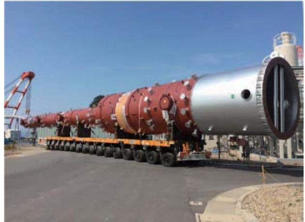
Fig. 17 (a) Transport of CO<sub>2</sub> absorber (October, 2018)
