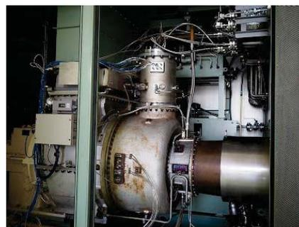
Fig. 3 Appearance of 2MWe Gas Turbine (IM270)
