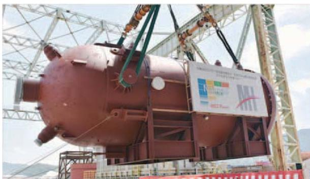
Fig. 6 Coal gasification furnace pressure containers
