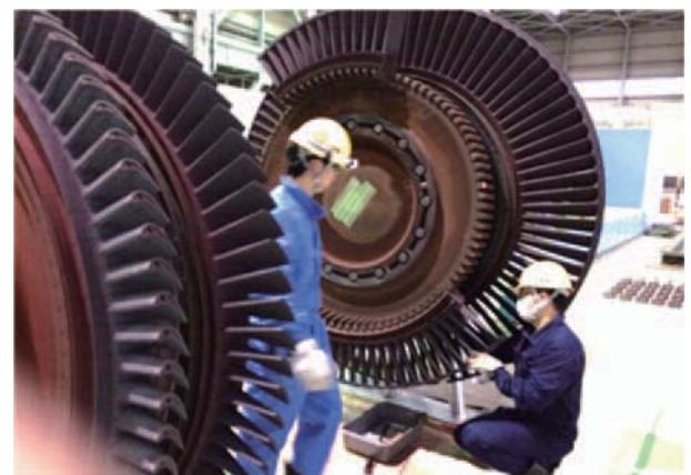
Fig. 15 (b) Inspection of gas turbine
