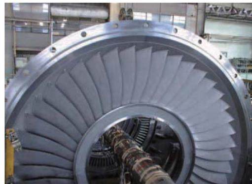
Fig. 10 "Inclined/radial" stationary blade
