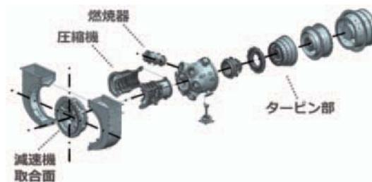
Fig. 6 Casing structure
