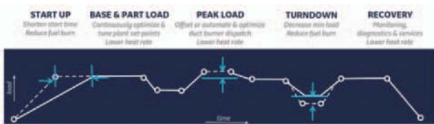
Fig. 10 Reduce fuel consumption during operations and with performance recovery
