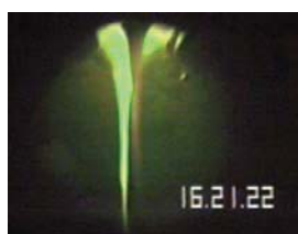
(b) Direct photo of slag flow in experiment
