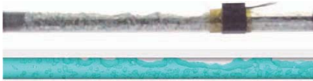
Fig. 13 Visualization of a boiling flow in a transparent cylindrical tube by electrical heating (upper) and corresponding simulation (lower).
