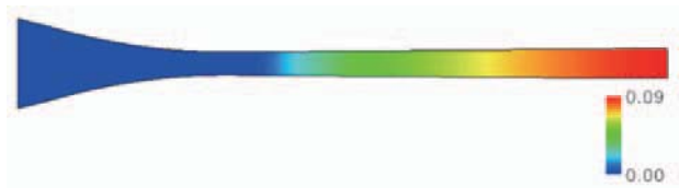
Fig. 11 Simulated mass fraction of CO 2 liquid
