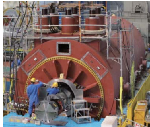
Fig. 15 Shop test of 900MVA indirect hydrogen-cooled turbine generator
