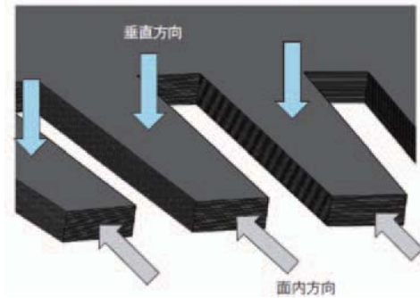
Fig. 11 Overview of magnetic flux flow to stator core experiment equipment
