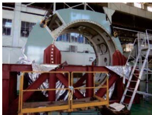
Fig. 7 Stator frame transportation style
