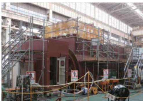
Fig. 5 Shop test of 500MVA class generator
