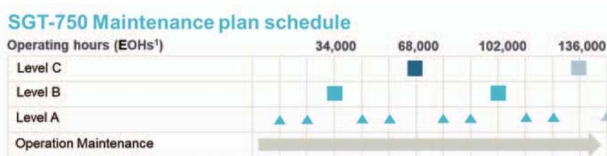
Fig. 9 SGT-750 Maintenance plan schedule (typical)
