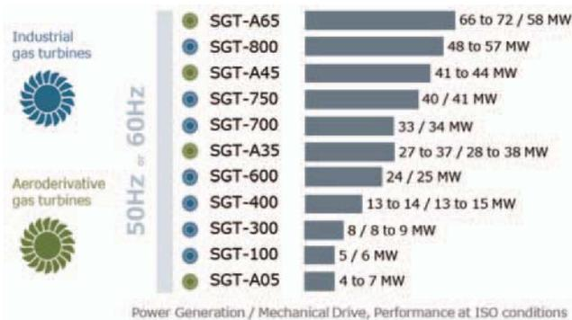
Fig. 2 Siemens gas turbine overview (Industrial & Aero derivative)
