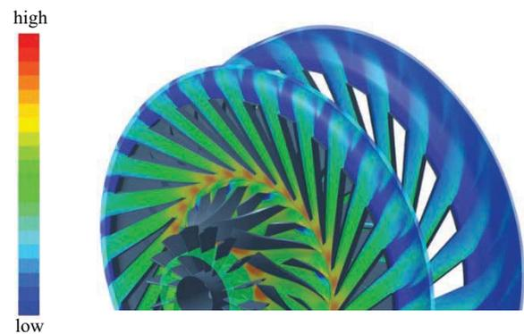
Fig. 2 Velocity distribution of 2-stage compressor model
