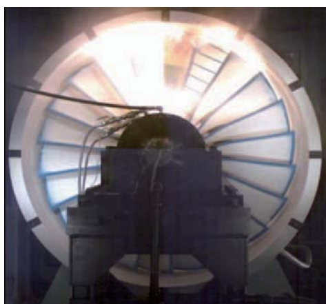
Fig. 12 FBO test (Containment rig test)
