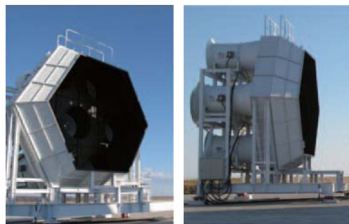
Fig. 13 Appearance of cross wind test equipment (Left: side Right: front)
