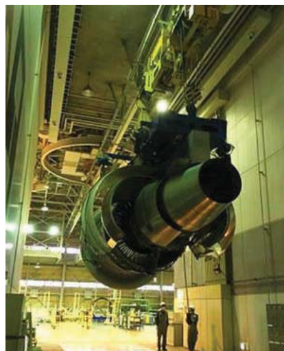
Fig. 6 Engine conveyed by crane
