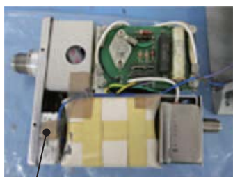
Thyristor Switching Element Outline Dimensions W150×H50×D130
