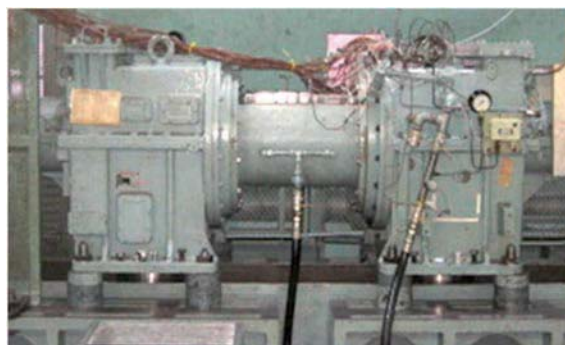
Fig. 11 The epicyclic gears on the power circulation type gear testing machine
