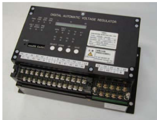
Fig. 14 Automatic voltage regulator
