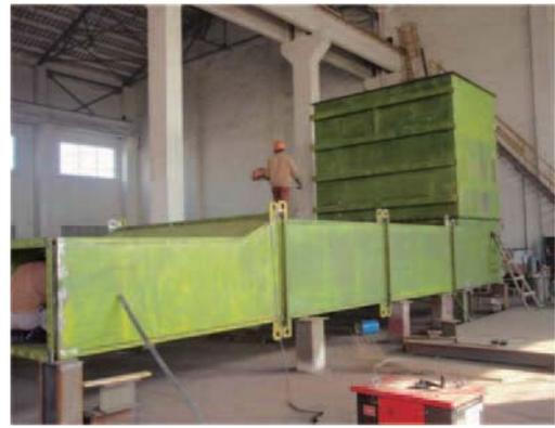
Fig. 13 Sample of GT intake duct
