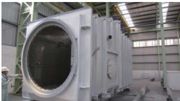
Fig. 17 Sample of Exhaust duct
