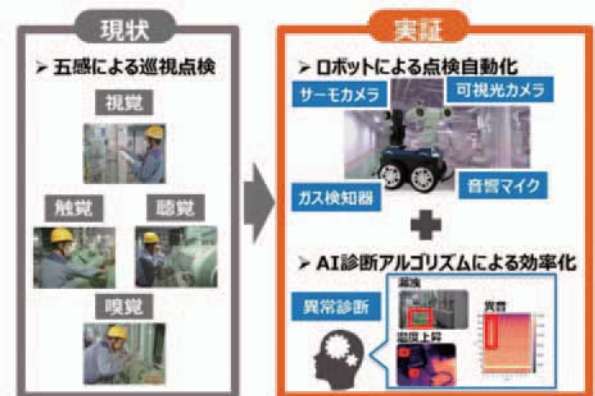
Fig. 5 Automatic inspection by robot
