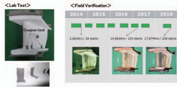
Fig. 9 Turbine row 1 vane advanced thicker TBC verification at t-point
