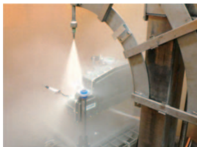
Fig. 14 High pressure water jet test
