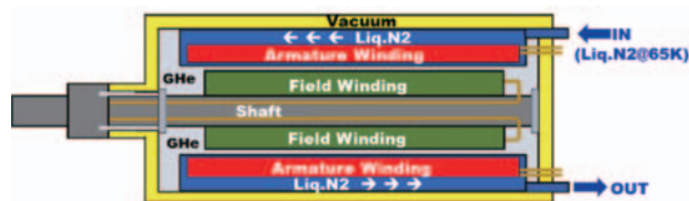
Fig. 6 Schematic drawing of cross-sectional view for proposing fully superconducting motor
