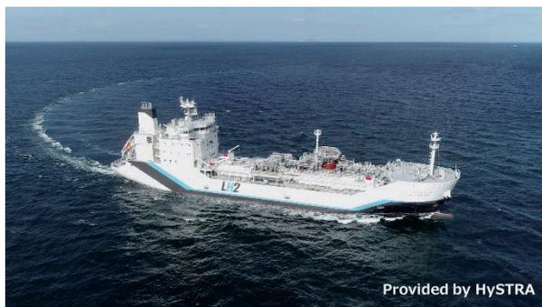
Fig. 4 Sea trial of liquefied hydrogen carrier "SUISO FRONTIER"
