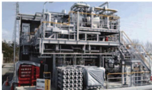
Fig. 3 Ammonia synthesis demonstration plant
