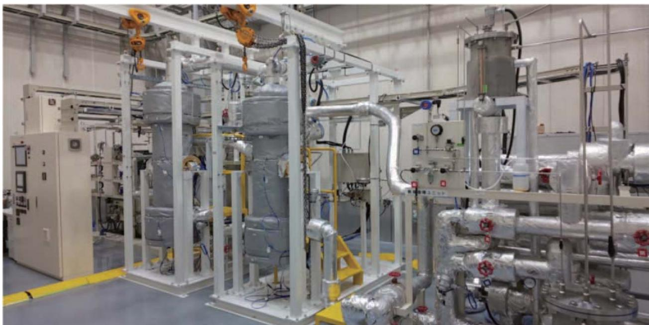
Fig. 10 Methanation bench test facilities
