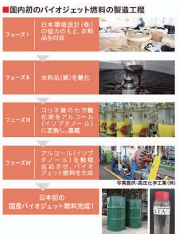
Fig. 3 Process to Produce SAF made from Cotton Clothes
