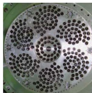
Fig. 5 Multi-cluster combustor (under development)
