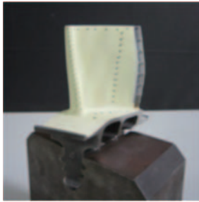
Fig. 2 Turbine blade with TBC
