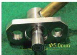
Fig. 19 Capacitive sensor<sup>(4)</sup>
