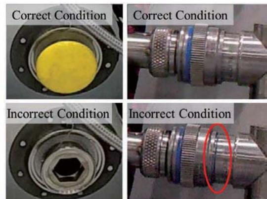
Fig. 6 Parts assembled and their defective portions
