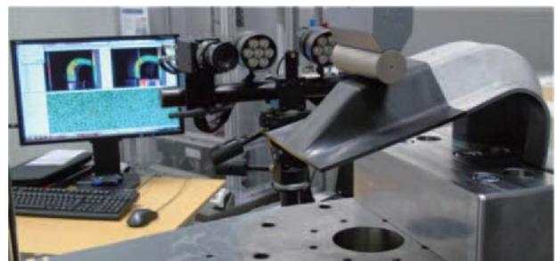
Fig. 17 Test setup for fiber-reinforced PA6 plastic parts
