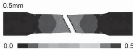
Fig. 5 Contour plots of the equivalent plastic strain distribution after fracture by SPG
