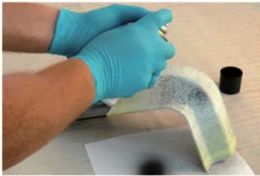
Fig. 10 Surface preparation with a stochastic pattern
