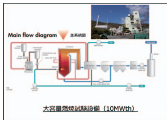
Fig. 5 Air and gas system in combustion test furnace and ammonia supply system overview (2)
