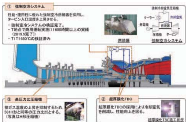
Fig. 4 Design Features of M501JAC gas turbine.
