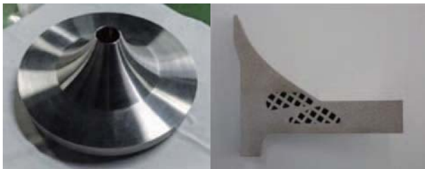
Fig. 19 Test disk and cross section by AM
