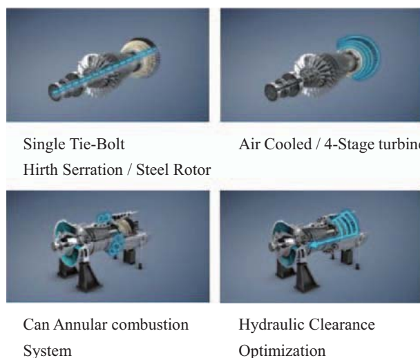
Fig. 3 Common Siemens Energy H- and HL-class design features (7)
