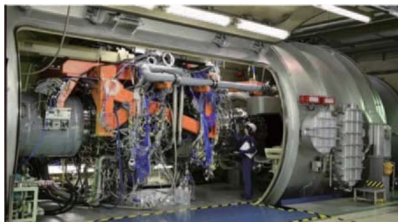
Fig. 16 Altitude test for XF9 at CTC ATF
