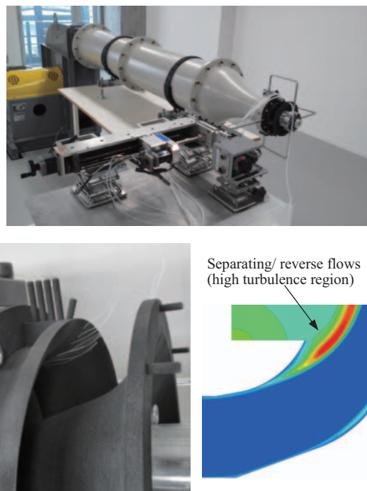
Fig. 5 The Low-speed wind tunnel and an exhaust hood model (upper), flow visualization test with tufts (lower left) and a CFD result (turbulence energy contours) (lower right)
