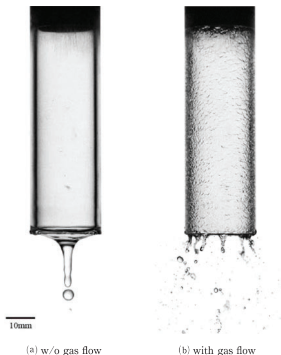
Fig. 5 From liquid film to droplet dispersion
