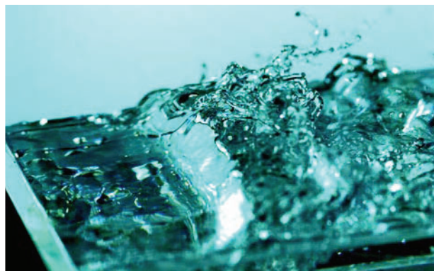
Fig. 3 Wavy liquid film sheared by fast gas flow
