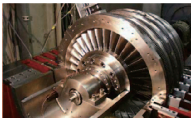
Fig. 2 Multi-stage compressor (3.5stages).
