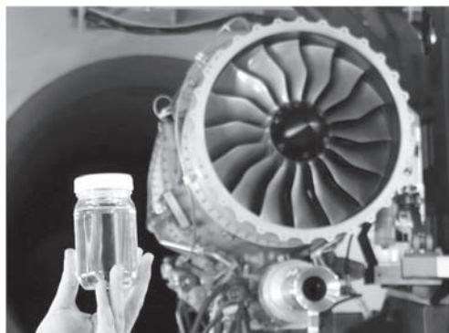
Fig. 7 HF120 engine test facility and SAF used in the test
