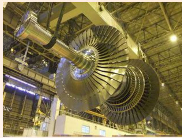
48" LP-rotor for Combined Cycle Steam Turbine by TOSHIBA ESS
