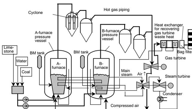
Fig.1 Conceptual diagram of PFBC system
