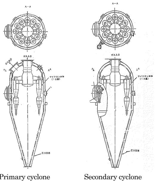
**Fig. 4 Cross section of cyclone-type dust collector**
