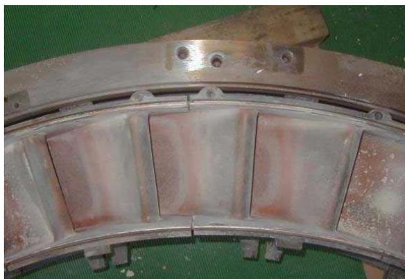
Fig. 6 Gas turbine first stage nozzle assembly
