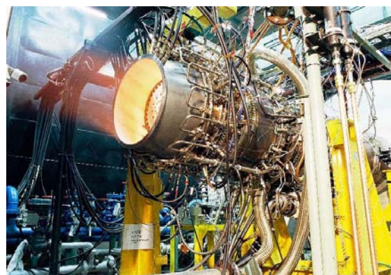
Fig.4 ESPR HTCE engine test
