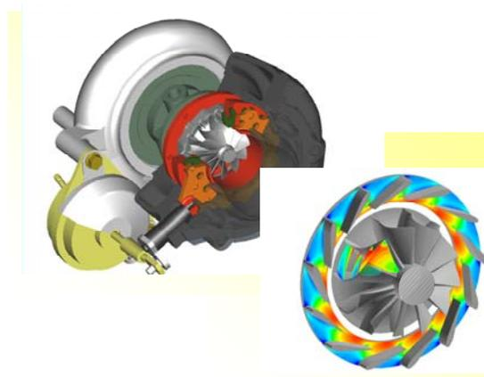
Fig.1 VG Turbo for passenger cars
