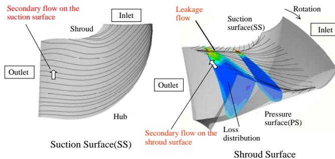
Fig.3 Arising loss mechanism in turbine blades (CFD result)
