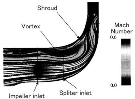
Fig.4 Surge vicinity flow analysis results for compressor impeller
