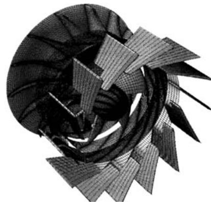
Fig.5 Casing treatment with vanes
