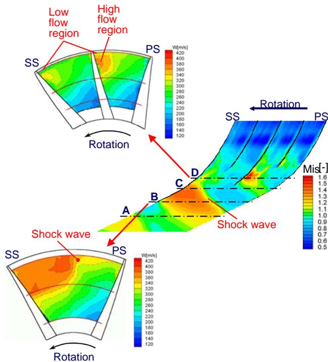
Fig.6 Measurement results of transonic compressor impeller
