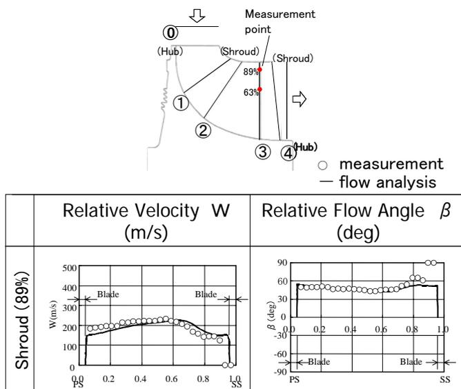
Fig.2 Comparison between measurement and flow analysis (radial turbine)
